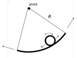
(a) Find the differential equations of motions that describe the angular displacement of the hoop and the swing. You may assume  $a/R \ll 1$  and small displacements from equilibrium.
