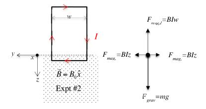
(a) In experiment #1, the only force acting is the constant force mg due to gravity, and the frame falls to earth just as a point mass m. That is, its velocity increases linearly, displacement quadratically in time.  $v_{B=0}(t) = v_0 + gt$ ;  $z_{B=0}(t) = z_0 + v_0 t + \frac{1}{2}gt^2$ . The right-handed system of axes above is set up so that increasing z is in the direction of travel.
