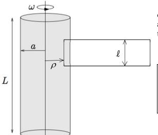
(c) Ampere's law with a rectangular loop with one arm *inside* the cylinder, using the same arguments as in (b), only now there *is* current threading the loop:
