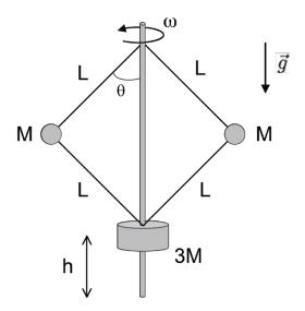
A flyball governor is a device commonly used in steam engines to control the flow of steam. In the simplified version shown above, a rotating shaft is connected to two hinges of mass M through rigid, massless rods of length L. The rods are also attached at the bottom of the device to a larger block of mass 3M which can slide freely up and down the shaft. The shaft rotates at constant angular rate  $\omega$ .
