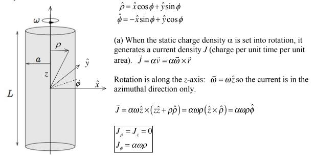
The task is to find the magnetic field *B*, which requires Ampere's law. First note that all the possible field components could in principle be functions of *z*,  $\rho$ ,  $\phi$ :
