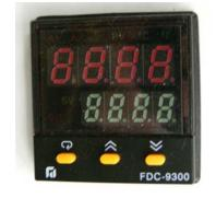
referred to as the SV or (Set-point Value.) To adjust the SV press either the up or down key until the lower display
