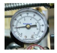
Please record the system pressure at the start-up of your Haskris system. Whenever the pressure increases 5-6 psi (0.3 - 0.4 Bar) above the initial start-up pressure, you should clean the strainer.
