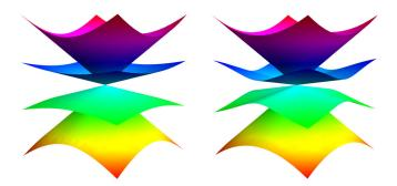
FIG. 1. Energy dispersion of the spin-3/2 Rarita-Schwinger-Weyl fermion at a fourfold linear band crossing point. We set one of the momentum components of p to zero and plot the eigenvalues of Eq. (1) versus the remaining two components for  $v_2 = 0$  (left) and  $v_2 = 1/3$  (right). For  $v_2 = 0$  the spectrum is rotation invariant, while for generic values of  $v_2$ , it features cubic anisotropy.
