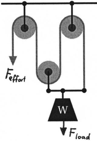
Mechanical advantage is defined as the ratio  $F_{load}/F_{effort}$ . What is the mechanical advantage of the pulley system illustrated above?
