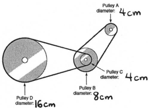
The figure shows a belt and pulley system. Pulley B and pulley C are rigidly connected. Pulley D is turned one full revolution. How many revolutions does Pulley A turn?
