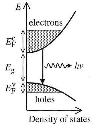
Fig. 5.7 Occupancy of the conduction and valence band states in the degenerate limit at  $T = 0$ . The electrons and holes have separate Fermi energies  $E_F^c$  and  $E_F^v$  respectively which are determined by the number of carriers injected into the bands. The conduction and valence bands are filled up to their respective Fermi levels, as shown by the shading.
