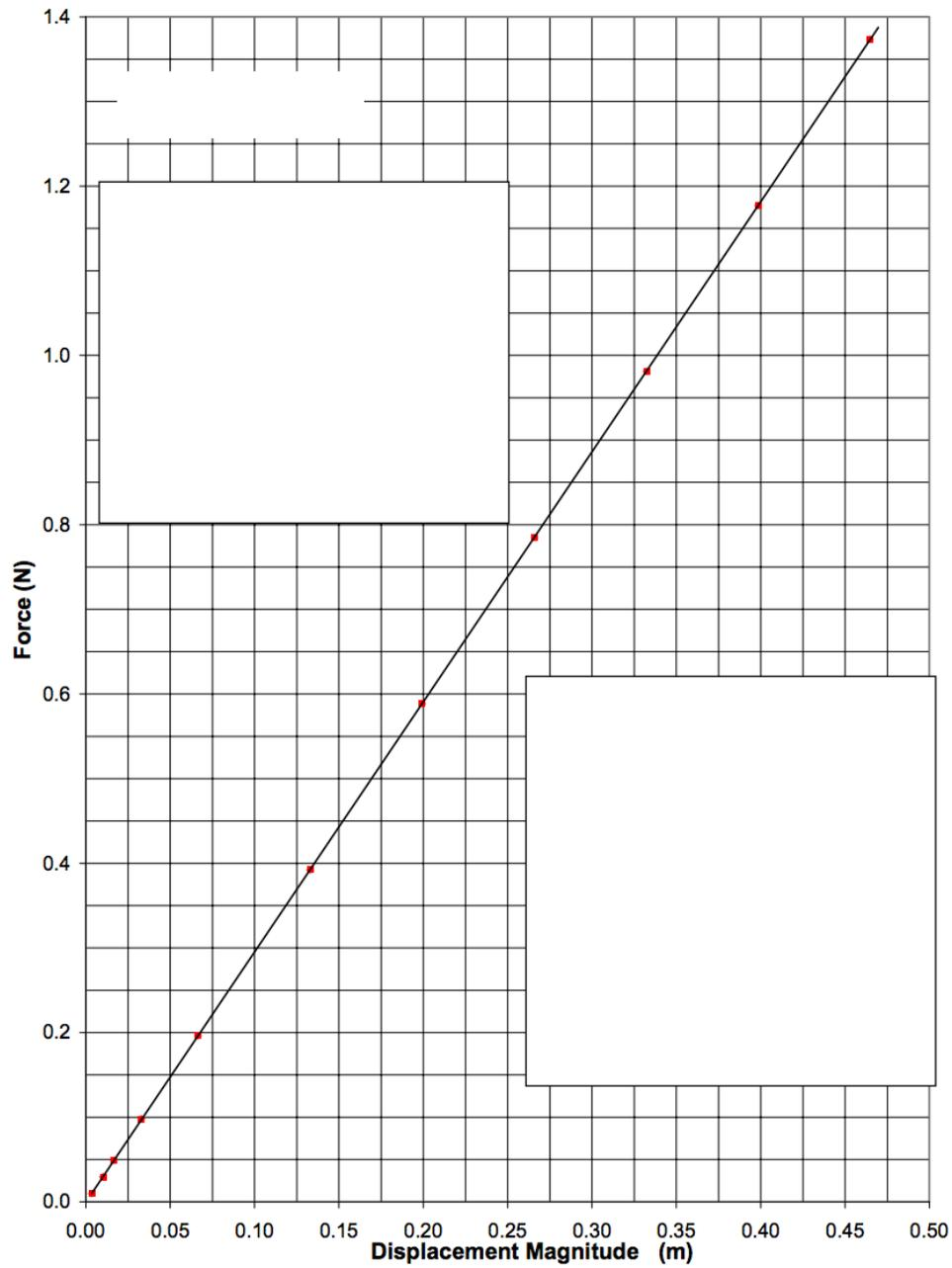
**Figure 2.** A plot of the downward force on the spring ( $mg$ ) as a function of the displacement of the spring,  $\Delta y$ .
