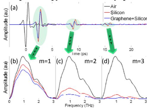
Fig. 4. (a) THz waveforms transmitted through air (black), silicon (red), and graphene on silicon (blue). (b-d) Amplitude spectra of the directly transmitted pulse ( $m = 1$ ) and the first two internally reflected pulses ( $m = 2$  and  $3$ ) through silicon (red) and graphene on silicon (blue). The spectrum of the pulse through air is added for comparison (Black line).
