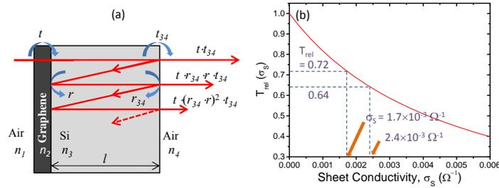
Fig. 3. (a) Multiple reflections at Air-Graphene-Si-Air interfaces:  $n_1 = n_4 = n_{\text{Air}} = 1$  and  $n_3 = n_{\text{Si}} = 3.42$ . (b) Relative THz transmission of graphene/Si versus sheet conductivity.
