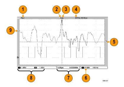
1. The acquisition readout shows when an acquisition is running or stopped. Icons are:
