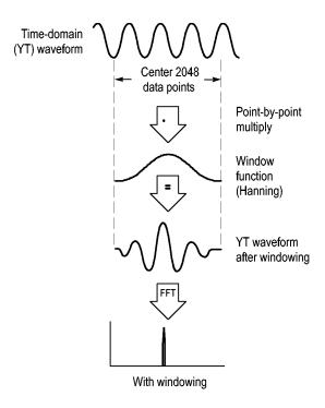
The FFT function includes three FFT Window options. There is a trade-off between frequency resolution and amplitude accuracy with each type of window. What you want to measure and your source signal characteristics will help you to determine which window to use.
