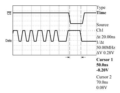
To set up to measure propagation delay, follow these steps:
