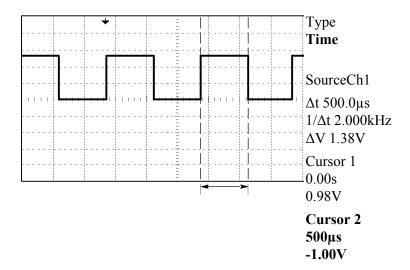
**NOTE.** The Positive Width measurement is available as an automatic measurement in the Measure Menu. See Measure on page 91.
