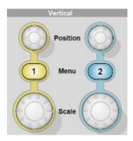
Position (1 and 2). Positions a waveform vertically.
