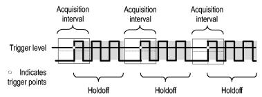
Triggers are not recognized during holdoff time.
