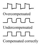
**4.** If necessary, adjust your probe. Repeat if necessary.
