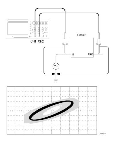
To view the input and output of the circuit in an XY display, follow these steps:
