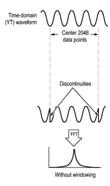
Applying a window to the YT waveform changes the waveform so that the start and stop values are close to each other, reducing the discontinuities.
