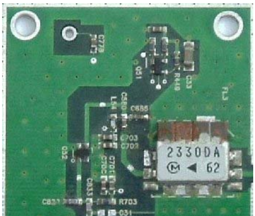
Fig. 1.3. A 4-pole Dielectric Resonator Filter for 2.4GHz, mounted on a pcb.
