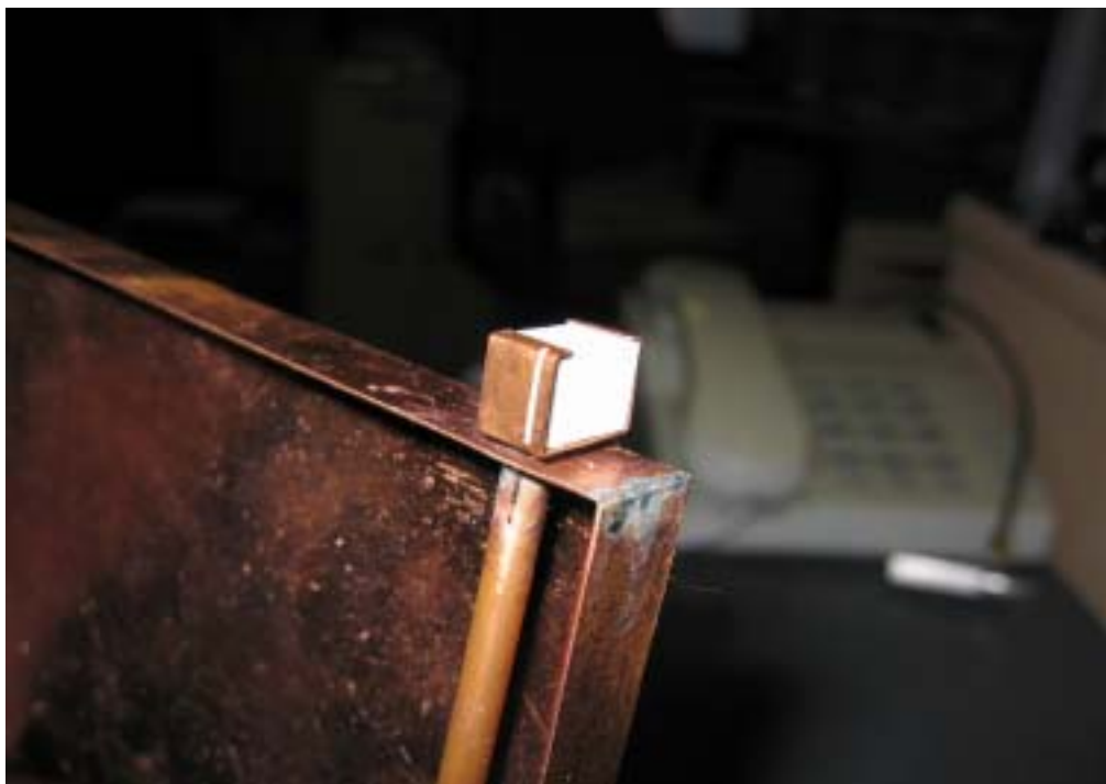
Figure 1.25: Antenna element (Size : 10mm x 5.5mm x 6.5mm)
