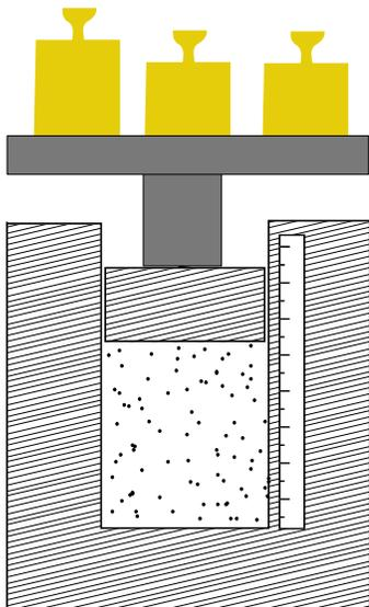
FIG. 2. Sketch of an experiment to measure the derivative  $\left(\frac{\partial U}{\partial p}\right)_S$  in Eq. 5. The piston is the same as that described in Fig. 2. As mentioned in the text, the procedure involves slowly adding weights to the top of the piston to change its pressure, and measuring the change in volume using a ruler. From this, the work is found, and from that the change in internal energy.
