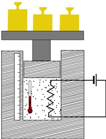
FIG. 6. Sketch of experiment to directly measure the derivative  $\left(\frac{\partial p}{\partial T}\right)_V$  in Eq. 15. The procedure involves heating the contents of an insulated piston with a resistor, and measuring how much weight needs to be added to the piston in order to return the system to its original volume.
