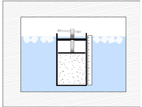
FIG. 5. Sketch of experiment to measure the derivative  $\left(\frac{\partial S}{\partial V}\right)_T$  in Eq. 10. A metal piston is inserted into an insulated container of ice water with a known quantity of ice. The volume of the piston is slowly changed, and afterwards the mass of the ice is measured.
