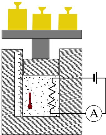
FIG. 7. Sketch of experiment to directly measure the derivative  $\left(\frac{\partial S}{\partial V}\right)_p$  in Eq. 16. The procedure involves heating the contents of an insulated piston with a resistor, while measuring the current (and thus power) and the temperature, and measuring the change in volume.
