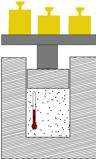
FIG. 1. Sketch of experiment to measure the derivative  $\left(\frac{\partial p}{\partial T}\right)_S$  in Eq. 2 by, in fact, measuring  $\left(\frac{\partial T}{\partial p}\right)_S$ . The procedure involves slowly adding weights to the top of the piston to change its pressure, having measured the area. The piston itself is insulated to keep the process adiabatic, and we use a thermometer inside to measure the resulting change in temperature.
