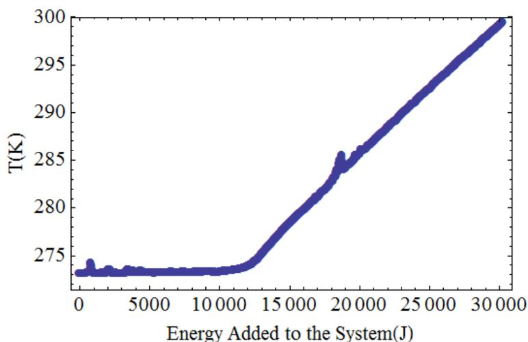
1. Find the latent heat of fusion, which is the amount of energy required to melt ice.
