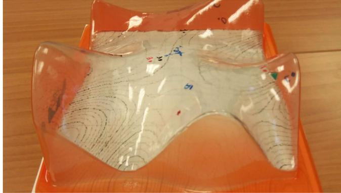
Figure 1: One of the transparent plastic surface models developed by Aaron Wangberg at Winona State University as part of the Surfaces project. Each of the six color-coded surfaces is dry-erasable, as are the matching contour maps, one of which is visible underneath the surface. For further details, see [26, 27].
