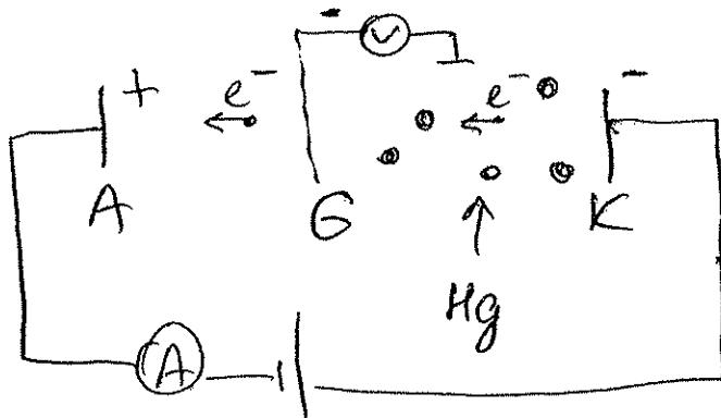
Triode filled with Hg vapor. Electrons are moving from K to A through a grid G, to which a small countervoltage is applied.
